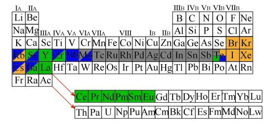
Figure 3.1: The chemical state of fission products, where orange denotes volatile fission products, grey denotes metallic precipitates, blue denotes oxide precipitates and green indicates products in solid solution. Elements labelled with more than one colour denote the possibility of an alternate chemical state, with the preferential chemical state denoted by the top colour.
