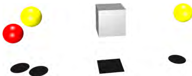
Figure 6.7: \text{O}_i^{\bullet} trapped by \text{Mg}_{\text{Al}}^{\bullet} . Yellow = \text{Mg}_{\text{Al}}^{\bullet} , grey = \text{V}_{\text{Mg}}^{\bullet} , red = \text{O}_i^{\bullet} .
