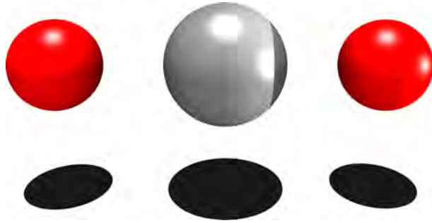
Figure 6.8: O''Mg_i^{••}O'' trimer. Grey sphere = Mg_i^{••} , red sphere = O'' .
