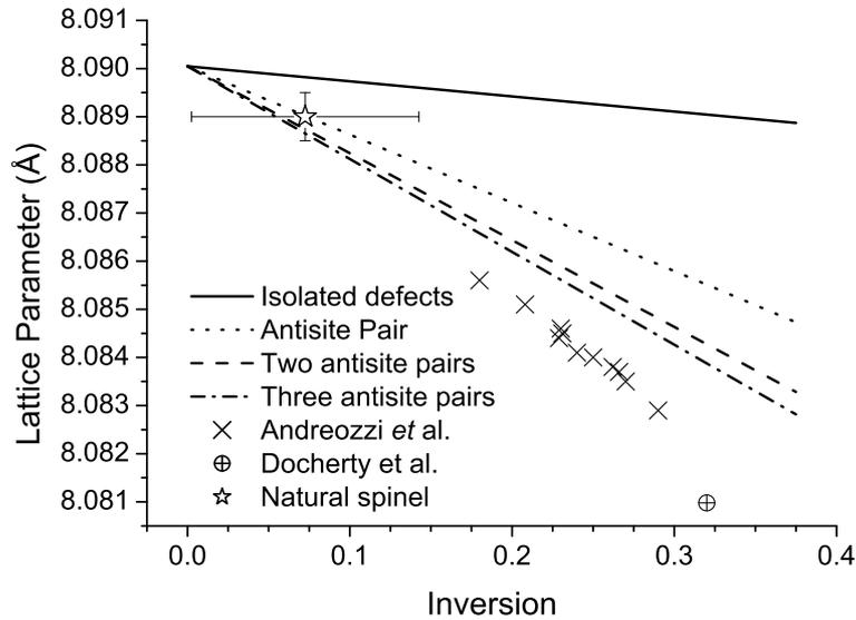
Figure 3.5: Variation in lattice parameter with inversion as predicted using defect volume analysis. The experimental data of Andreozzi *et al.* [117], Docherty *et al.* [118] and Hafner *et al.* [28] are included for comparison.
