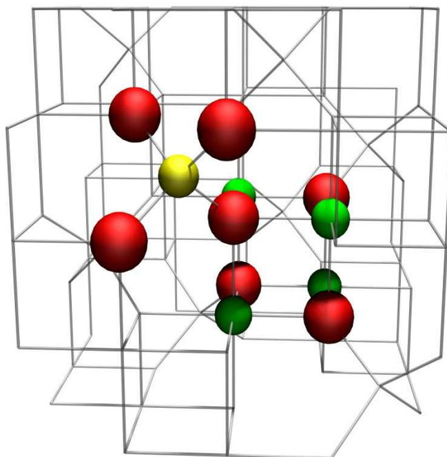
Figure 3.1: A single unit cell of normal  $MgAl_2O_4$  spinel showing a tetrahedral  $Mg^{2+}$  coordinated by four  $O^{2-}$  ions corner linked to a cube composed of four octahedral  $Al^{3+}$  and four  $O^{2-}$  ions.
