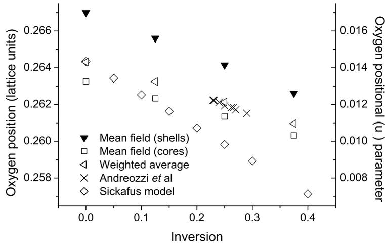
Figure 3.7: Variation in oxygen positional ( $u$ ) parameter with inversion predicted using a mean field analysis. Results are compared with experimental data [117] and the model of Sickafus *et al.* [38].
