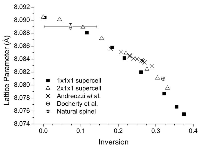
Figure 3.6: Variation in lattice parameter with inversion as predicted using CEMMC analysis. The experimental data of Andreozzi *et al.* [117], Docherty *et al.* [118] and Hafner *et al.* [28] are included for comparison.
