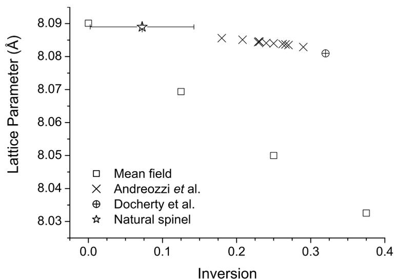
Figure 3.4: Variation in lattice parameter with inversion predicted using a mean field analysis. This shows significant deviation in slope from the experimental data [28, 117, 118].
