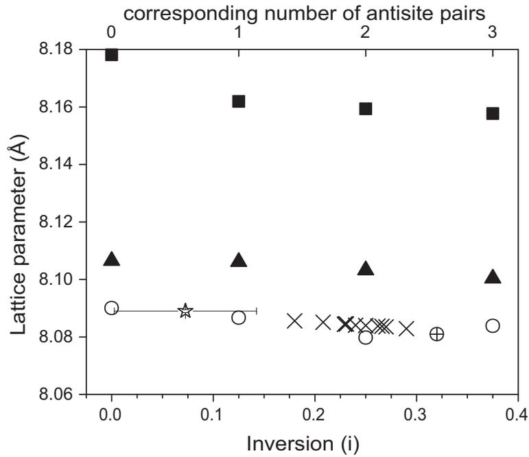
Figure 3.3: Variation in lattice parameter with inversion for specific defect cluster configurations containing, respectively, 0, 1, 2 and 3 antisite pairs. The solid square symbols correspond to GGA DFT calculations, the solid triangles to LDA DFT calculations, the open circles to pair potential calculations and the experimental data is represented as crosses [117], crossed circles [118] (synthetic samples) and by a star [28] (natural sample).
