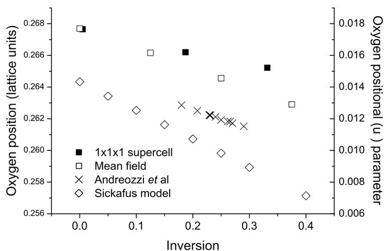
Figure 3.10: Variation in oxygen positional ( $u$ ) parameter with inversion predicted using the CEMMC and mean field methodologies. Oxygen ions are modeled without a shell. Results are compared with experimental data [117] and the model of Sickafus *et al.* [38].
