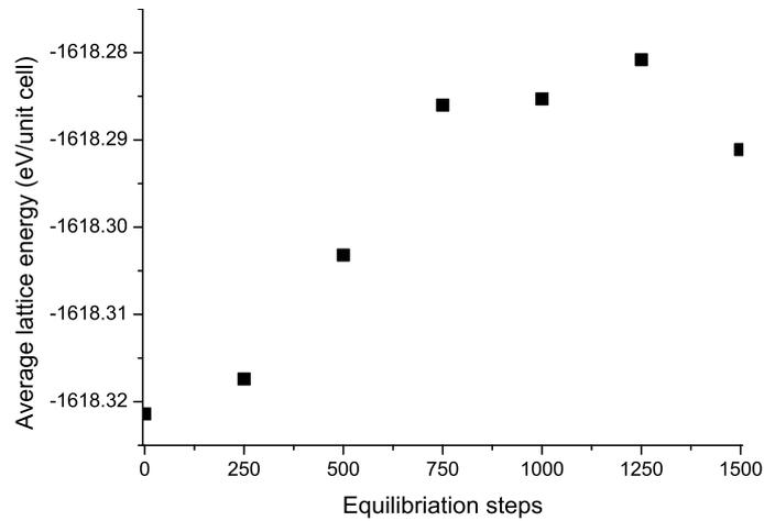
Figure 3.2: Mean lattice energy (eV) of a single unit cell of spinel over 6000 CEMMC swap attempts following the shown number of equilibration steps (at a target temperature of 2000K).
