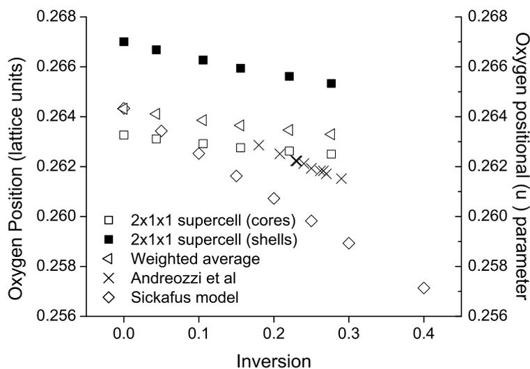
Figure 3.9: Variation in oxygen positional (u) parameter with inversion predicted using the CEMMC methodology with a 2x1x1 supercell. Results are compared with experimental data [117] and the model of Sickafus *et al.* [38].
